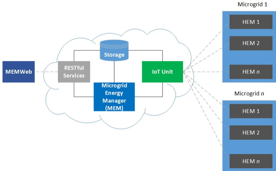
MEMCloud consists of five main components that include storage, RESTful Services, IoT Unit, Microgrid Energy Manager (MEM) and MEMWeb.
